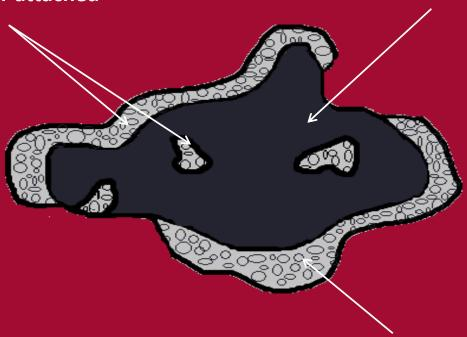
CO<sub>2</sub> enters the old mortar pores and makes it stronger
